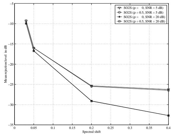
Fig. 5. Performance evaluation: Mean rejection level in dB versus spectral shift.
