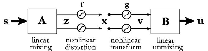
Fig. 1: Building blocks of the PNL mixing model and the separation system.
