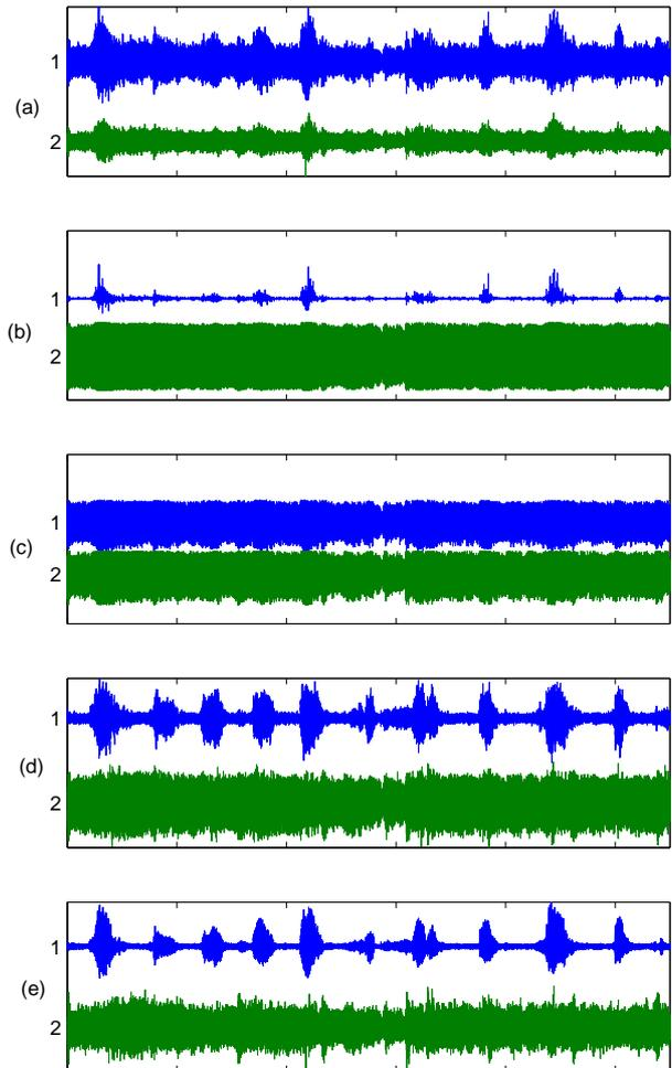
**Fig. 6:** Two channel audio dataset: (a) waveforms of the recorded (undistorted) microphone signals, (b) observed PNL distorted signals, (c) result of ACE, (d) recovered sources using ACE and a convolutive BSS algorithm and (e) for comparison convolutive BSS separation result for undistorted signals from (a).
